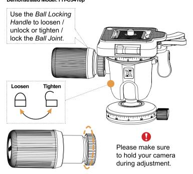
Friction can be adjusted by turning the *Friction Control* ring, simply pull out the handle then loosen the ring to reduce friction or tighten it to increase friction.
