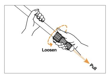
Turn in the direction shown to loosen the *Leg Locking Ring(s)*, pull out the leg section(s) to your desired length then turn the ring(s) in the opposite direction to tighten. The anti-rotational design enables you to loosen or tighten all *Leg Locking Ring(s)* simultaneously.
