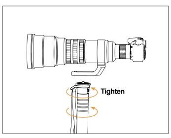
Locate your camera's screw hole or lens' connection socket, then insert the Mounting Screw into the screw hole / socket and turn the monopod until the camera / lens is firmly attached. Do not overtighten.
